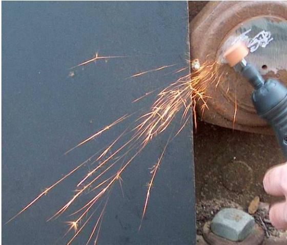
Figure A.3 Pin with 0.19% carbon content
