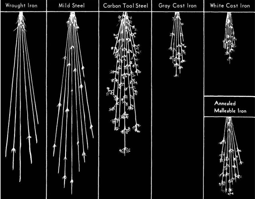
Figure A.1 Spark patterns for ferrous metals, Norton Abrasives
