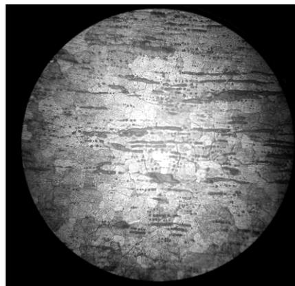
Figure 3. Field metallography (100x, nital etch) of 1881 wrought iron eyebar showing normal ferrite matrix and finely distributed slag.
