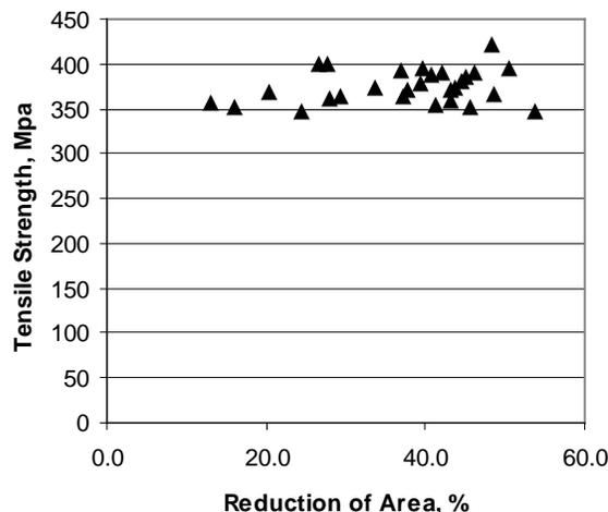
Figure 2. Tests of wrought iron (Holley 1877) based on Gordon 1988. While a lower bound for strength is easily determined, there is a widely scattered range of ductility as represented by reduction of area.
