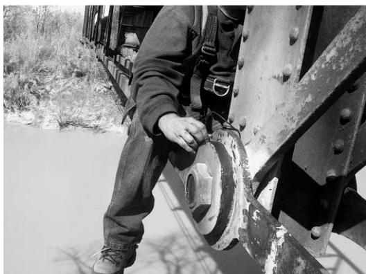
Figure 3. Circumferential ultrasonic testing of critical eyebar on 1896 Steel Truss Bridge
